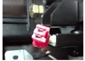
Now you can wrap a bit of adhesive tape on thread of the sensor and place it back where it was.
