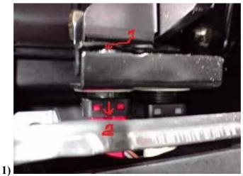
Place your screwdriver into position between metal guard and brake pedal like in pic red marker no.1 and lift it to get plastic bolt out of there the way of no.2. Don't worry, it holds on two wires and wont fall down anywhere. Now when you Provided by 406 Coupe Club got it free from bracket http://www.406coupeclub.org
